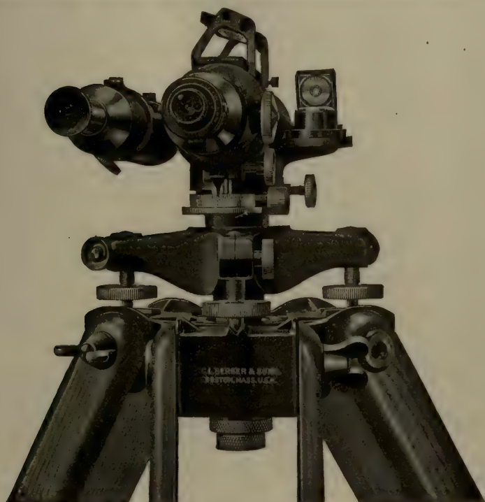
FIG. 89a. Precise Level. (C. L. Berger and Sons.)
